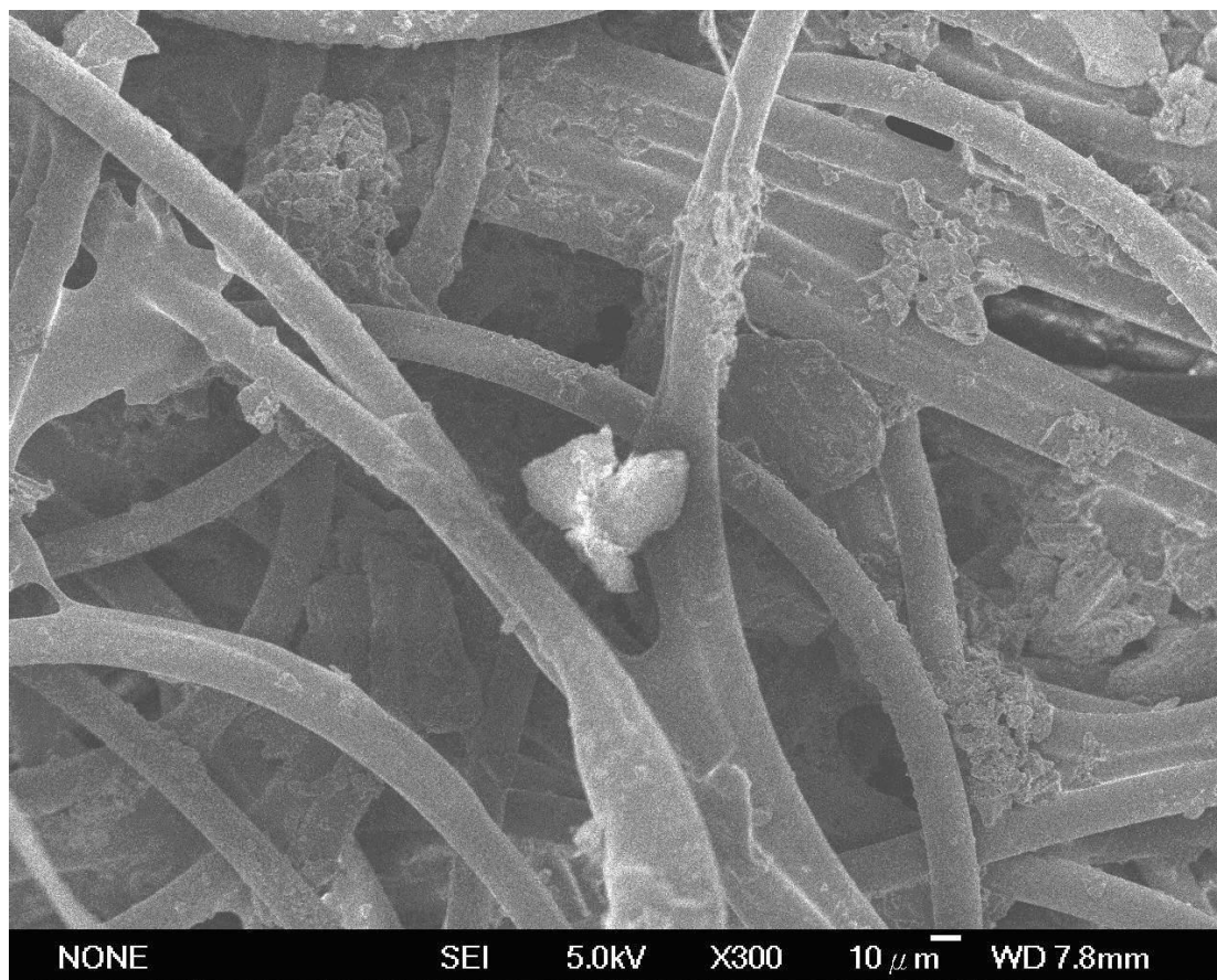
Figure 2. The SEM image of non-woven fabrics processed in 5% resin, 20 g/L bamboo charcoal (x250).
