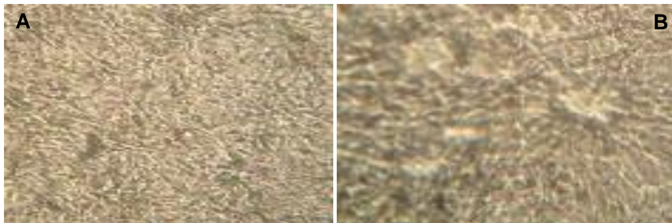
Figure 7. Surface structures of polyethylene films on microscope. (A) Without cell inoculation; (B) With cell inoculation NDYS-4.
