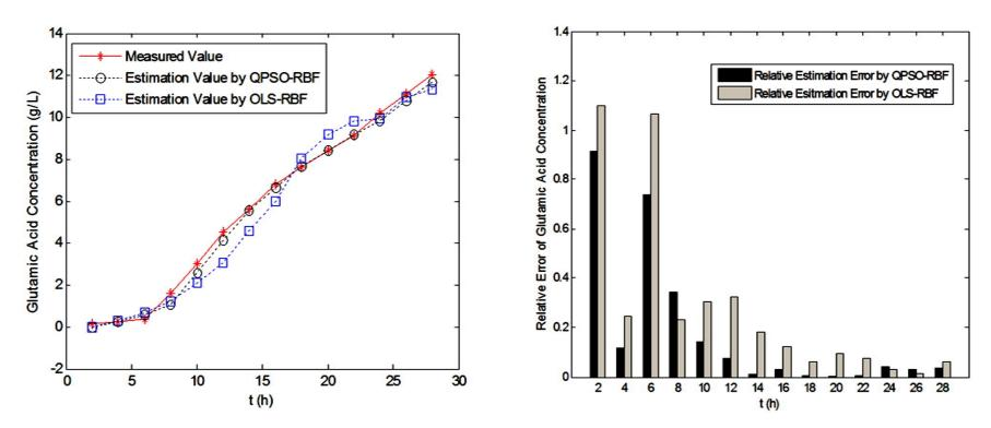
Figure 4. Estimation curves and relative estimation errors for the glutamic acid concentration generated by QPSO-RBF and OLS-RBF.
