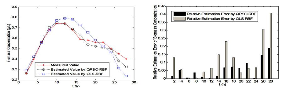
Figure 3. Estimation curves and relative estimation errors for the biomass concentration generated by QPSO-RBF and OLS-RBF.
