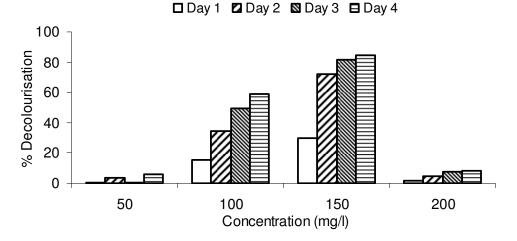
Figure 3. Effects of different concentration of Reactive Blue 2 on decolourisation by sulphate reducing bacteria in untreated sludge.
