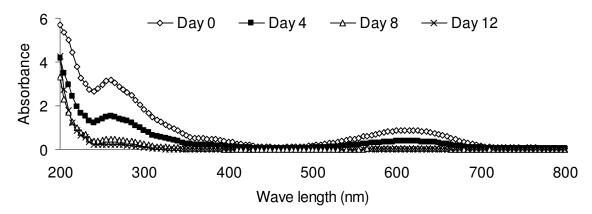
**Figure 1.** Typical changes in absorbance peaks monitored in a bioreactor for the anaerobic degradation and decolourisation of Reactive Blue 2 (100 mg/l) by sulphate reducing bacteria in untreated sewage sludge.
