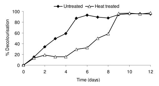
**Figure 2.** Percent decolourisation of Reactive Blue 2 (100 mg/l) dye by sulphate reducing bacteria grown in untreated sludge and heat treated sludge over 12 days.
