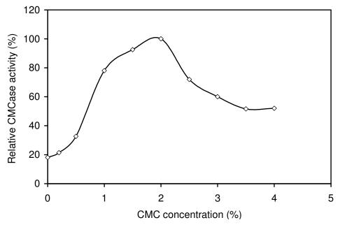
**Figure 5.** Effect of CMC concentration on endoglucanase production by *A. awamori* VTCC-F099. The endoglucanase activity was determined with 0.5% CMC in 0.1 M potassium phosphate buffer pH 6.5 at 30 °C.
