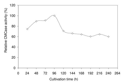
**Figure 2.** Time course of the endoglucanase production by *A. awamori* VTCC-F099. The endoglucanase activity was determined with 0.5% CMC in 0.1 M potassium phosphate buffer pH 6.5 at  $30\,^{\circ}$ C.
