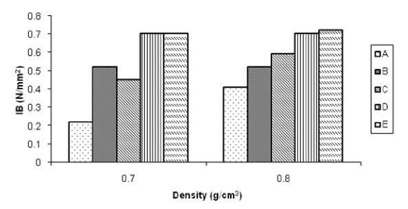
Figure 7. Internal bond strength of panels.
