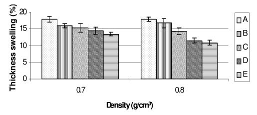
Figure 2. The 24 h thickness swelling of the panels.
