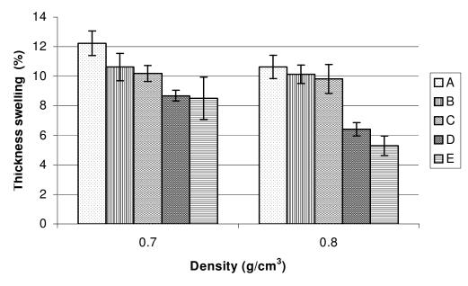
Figure 1. The 2 h thickness swelling of the panels.
