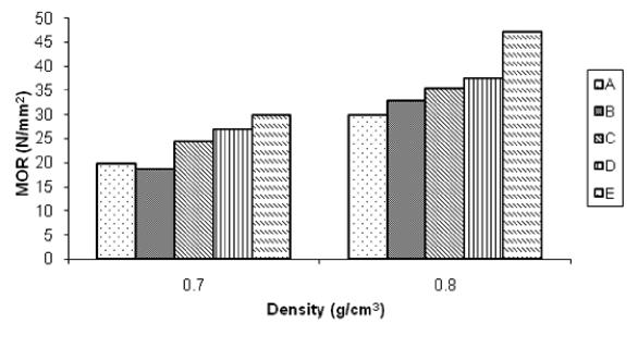
Figure 5. Bending strength of panels.
