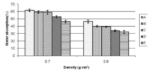
Figure 4. The 24 h water absorption of the panels.
