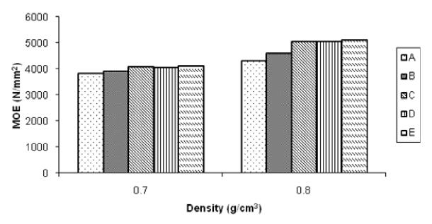
Figure 6. Modulus of elasticity of panels.
