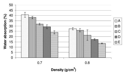
Figure 3. The 2 h water absorption of the panels.
