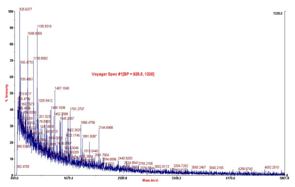
Figure 2. The molecular weight distribution of PSB was measured by a mass spectrograph; PSB was obtained by fermentation of swine blood with A32, micro-filtration, ultra-filtration, and spray-drying.
