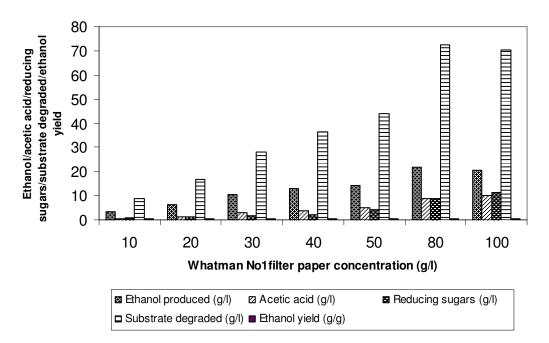
**Figure 4.** Coculture fermentation of high concentration of Whatman No 1 filter paper to ethanol by *C. thermocellum* CT2 with *C. thermosaccharolyticum* HG8.
