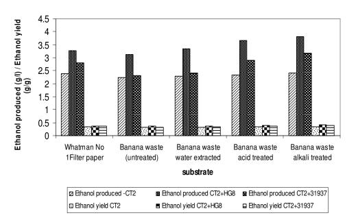
**Figure 2.** Ethanol produced and ethanol yields in mono and coculture fermentations of banana leaves by *C. thermocellum* CT2 with HG8 and ATCC 31937.
