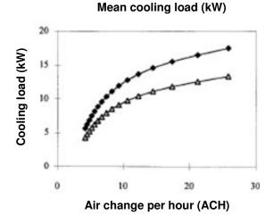
**Figure 7.** Cooling load by night ventilation for desired room indoor air temperatures of 23 and 25°C.
