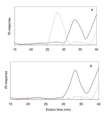
**Figure 5.** Analysis of the action mode of *B. senegalenis*  $(1\rightarrow3)$ -B-D-glucanase par HPSEC. A) hydrolysis products of laminarin. B) Hydrolysis products of insoluble yeast glucans. Incubations were performed in 100 mM sodium acetate buffer pH 4.5 at 40 °C, fort 30 min.(----) Substrate alone, (---) substrate + enzyme.
