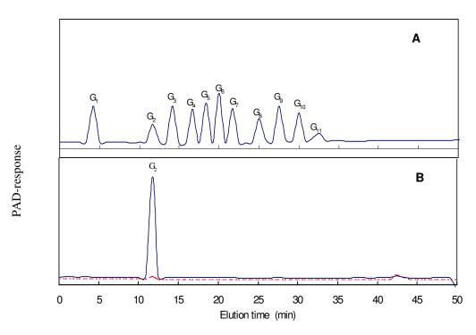
**Figure 4.** HPAEC elution patterns of hydrolysis products of raw starches by *G. klattianus* β-amylase. (----) substrate alone, (—) substrate + enzyme. (A). Elution profile of maltodextrin standards. (B). elution profiles of the incubation mixture of the enzyme with the substrate.
