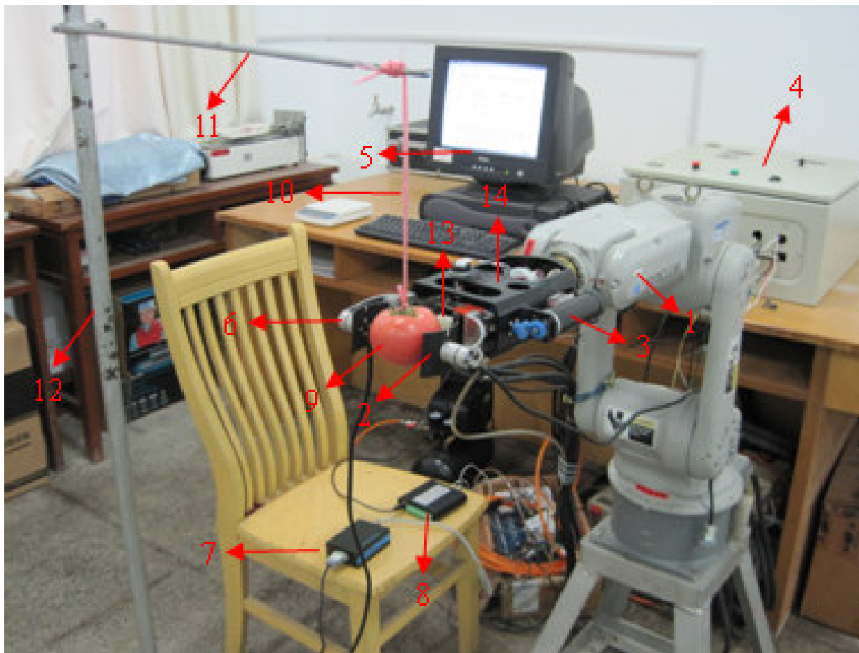
Figure 1. Experimental system. 1: tomato-harvesting robot; 2: finger; 3: motor; 4: control cabinet; 5: computer; 6: pressure sensor; 7: signal amplifier; 8: USB5935 data acquisition instrument; 9: tomato; 10: string; 11: beam; 12: height-adjustable stand 13: sucker; 14: end-effector.
