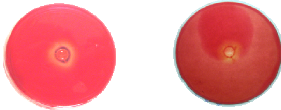
Figure 1. Yellow color area in centre of substrate agar plate shows the hydrolysis of carboxy methyl cellulose by endoglucanase activity.
