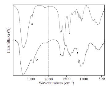
Figure 1. FTIR of NSC (a) and chitosan (b).
