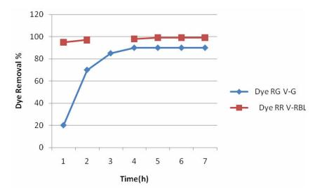
**Figure 2.** Kinetics of dye removal by PAC (1.5 gl<sup>-1</sup>) at concentration of residual dye in water after coagulation treatment (0.012 gl<sup>-1</sup> RR V-RBL and 0.010 gl<sup>-1</sup> RG V-G).
