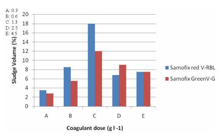
**Figure 1.** The volume of sludge formed at maximum removal of RR V-RBL and RG V-G using different coagulant doses
