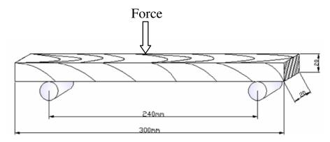
Figure 1. The dimensions of bending strength test specimens.
