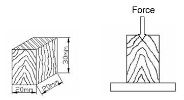
Figure 2. The dimensions of pressure strength test specimens.
