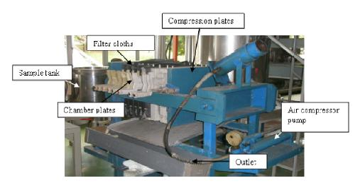
Figure 1. A Mechanical Filter Press used in the present study.
