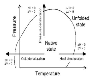
**Figure 7:** Typical phase transition curve of proteins in the PTdiagram. The relation between heat, cold and pressure-denaturation of proteins is presented by the sign of enthalpy changes ( $\Delta$ H) and volume changes. ( $\Delta$ V), Redrawn from Heremans (2002).
