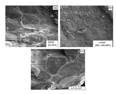
**Figure 19.** Micrographs of high-pressure frozen gelatin samples. (a) High-pressure assisted freezing under 50 MPa. (b) High-pressure shift freezing from 350 MPa/-17°C to 50 MPa. (c) an air-blast frozen gelatin sample (air temperature: -40°C, air speed: 5.5 m/s).
