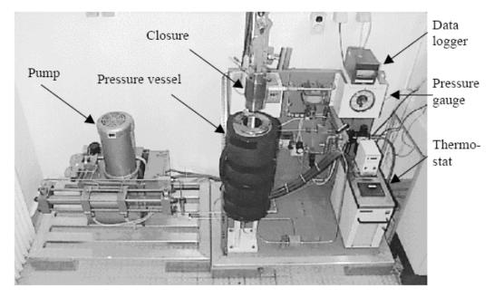
**Figure 1.**A lab-scale high hydrostatic pressure system. The maximum pressure of the system is 600 MPa with a filling volume of 0.6 L, Temp.: 0 ℃ to 95 ℃ (National Forge Europe, Belgium).Redrawn from (Dong-Un Lee ,2002).
