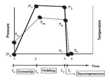
**Figure 4.** Typical variables (pressure, temperature, and time) to indicate conditions of HPP testing. Ambient pressures Ps and Pf are typically 0.1 MPa. Tm is the maximum temperature at process pressure. The difference between ambient temperatures before and after high-pressure processing. (Ts and Tf) generally indicates the extent of heat loss during testing (with the assumption that the depressurization time is within a few seconds). Redrawn from Balasubramaniam et al 2004
