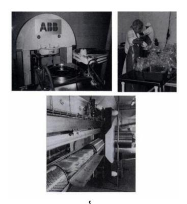
**Figure 5.** High pressure production of avocado product(A) installed high pressure autoclave at Avomex .Inc.(New Mexico).(B) preparation of avocado paste at Avomex.(C)high pressure processing of cooked ham at Espuna SA,CO, in Olot. Spain. (Redrawn from Hendrickx et al., 2005b.)
