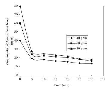
Figure 11. Degradation of 2,4-dichlorophenol by immobilized crude extracts of *Mycoplana dimorpha* (combination 27).
