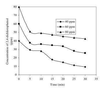
Figure 7. Degradation of 2,4-dichlorophenol by immobilized crude extracts of *Mycoplana dimorpha* (combination 15).
