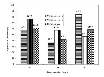
Figure 13. Degradation of 2,4-dichlorophenol by immobilized crude extracts of *Mycoplana dimorpha* (combinations 12,15 and 18).
