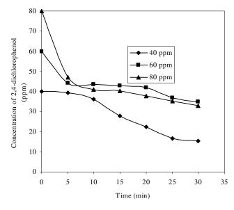
Figure 8. Degradation of 2,4-dichlorophenol by immobilized crude extracts of *Mycoplana dimorpha* (combination 15).
