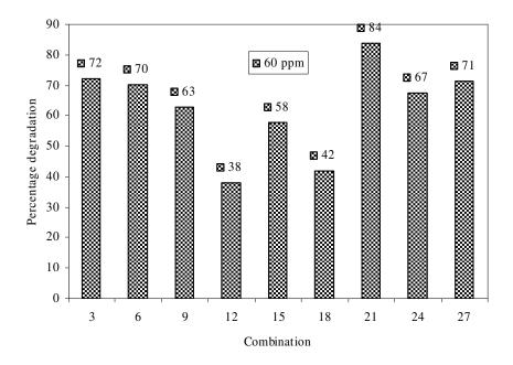
Figure 16. Degradation of 2,4-dichlorophenol using immobilized crude extracts of *Mycoplana dimorpha* (60 ppm).
