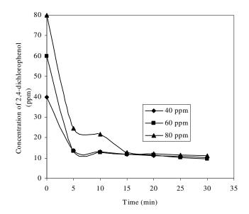
**Figure 9.** Degradation of 2,4-dichlorophenol by immobilized crude extracts of *Mycoplana dimorpha* (combination 21).
