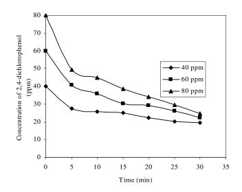
**Figure 5.** Degradation of 2,4-dichlorophenol by immobilized crude extracts of *Mycoplana dimorpha* (combination 9).
