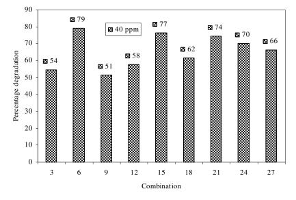
**Figure 15.** Degradation of 2,4-dichlorophenol using immobilized crude extracts of *Mycoplana dimorpha* (40 ppm).
