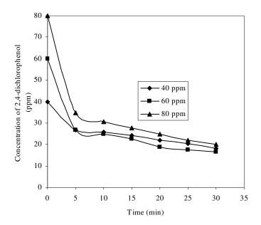
Figure 3. Degradation of 2,4-dichlorophenol by immobilized crude extracts of *Mycoplana dimorpha* (combination 3).
