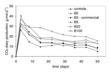
**Figure 5.** Daily CO<sub>2</sub> production during incubation of the respirometric experiment with the water contamination.
