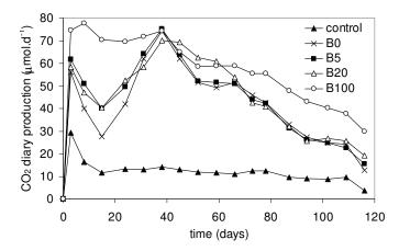
**Figure 1.** Daily CO<sub>2</sub> production during incubation of the first respirometric experiment with the soil contamination.
