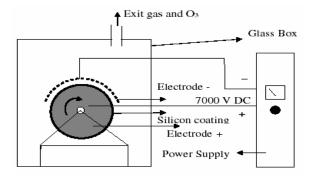
Figure 1. Main components of corona reactor.
