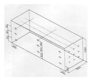
Figure 1. Measuring points of compost temperature.
