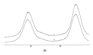
Figure 2. X-ray pattern of cellulose produced by *Gluconacetobacter xylinum* ATCC 10245 from a. glucose medium b. molass medium.
