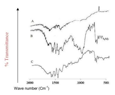
Figure 1: FTIR spectra of isapgol husk (A), diclofenac sodium (B) and formulated tablet (C)
