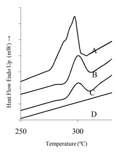
**Figure 2:** DSC thermograms of diclofenac sodium (A), physical mixture of diclofenac sodium and husk (1:1) (B), batch 4 tablet (C) and isapgol husk (D).
