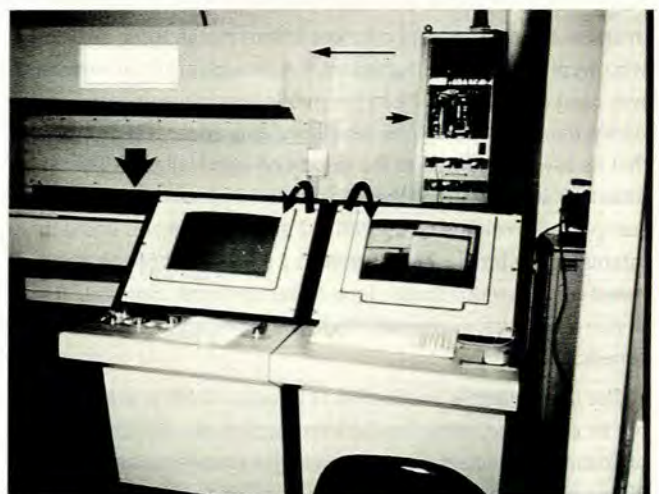
Fig. 1. Components of the 'Modified Scannex' digital radiography unit, showing user console with viewing and operating display monitors (curved arrows). The patient bed (broad arrow), scanner housing (long arrow) and electronics cabinet (short arrow) are also seen.
