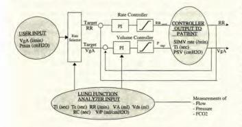
Fig. 1. Diagram of the ALV controller showing the input and output relationships. User input is V<sup>2</sup>gA (I/min) and Pmax (cm H<sub>2</sub>O). Lung function analyser input is Ti (s), Te (s), RR (/min), VA (ml), Vds (ml), RC (s) and V/P ratio (ml/cm H<sub>2</sub>O). Controller output is mandatory rate (/min), Ti (s) and Pinsp (cm H<sub>2</sub>O). (From Chest.<sup>3</sup>)
