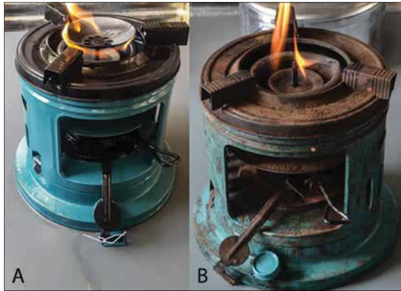
Fig 1. (A) New paraffin stove – note the fuel leak. (B) In-use stove, with a damaged self-extinguishing mechanism and flame snuffer.
