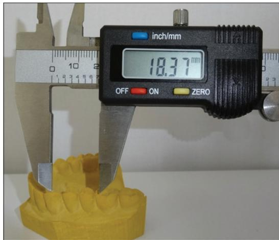
**Figure 3:** Linear measurements with digital calipers on the plaster model
