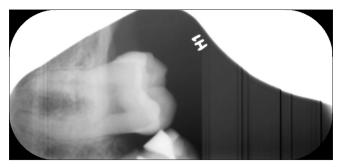
Figure 9: A physically damaged plate due to scratching
