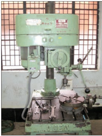
Figure 1: Radial drilling machine used for drilling the master cast at specified angulation
