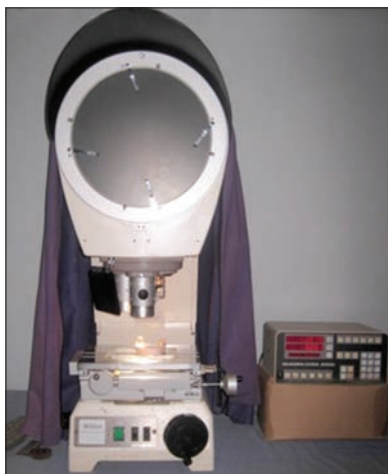
Figure 3: Profile projector and image of implant analog as seen on the projector screen
