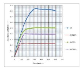
**Fig. 1:** Change in turbidity with time course measured by variation in absorbance at 620nm with and without inhibitor (BDE); various curves showing the percentage inhibition of calcium oxalate crystallyzation with BDE with respect to control.
