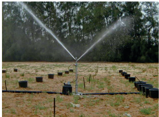
Figure 1 Measuring of sprinkler base pressure
