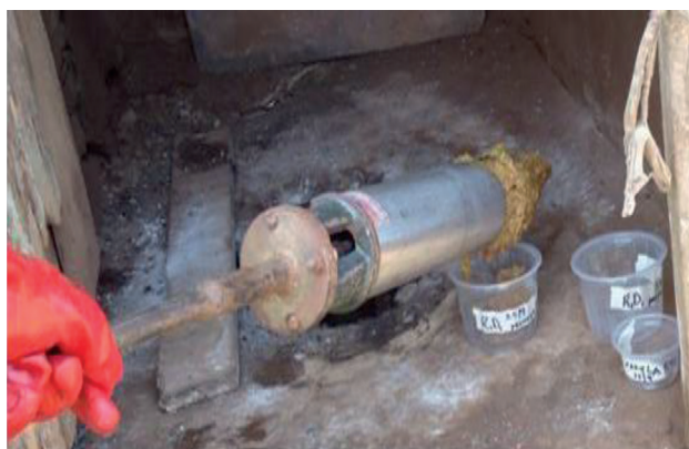
Figure 2 Pit latrine sludge sampling using a sludge sampler
