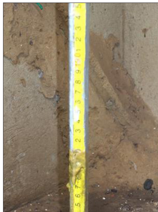
Figure 4 Depth tool with sludge markings (Makerere University, 2015)
