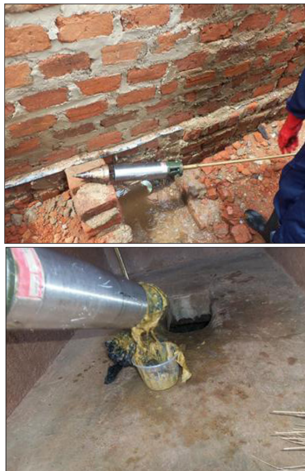
Figure 3 Pit sludge sampler (Makerere University, 2015)
