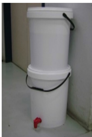
Figure 4 (a) Schematic diagram; and (b) photograph of the bucket filter (BF)
