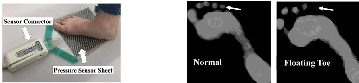
(a) Method for measuring foot pressure distribution (b) Left: normal foot pressure distribution; Right: fifth toe floating
