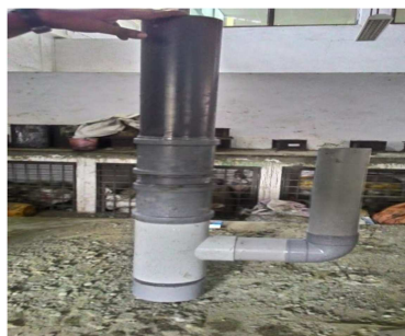
Fig. 7 Falling head permeameter used for permeability testing
