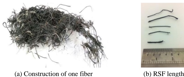
Fig. 1 The RSF extracted from waste tires
