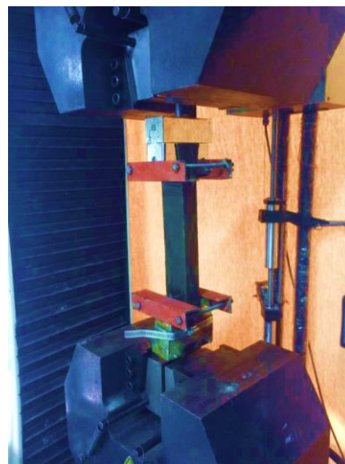
(b) Uniaxial tensile tests setup
