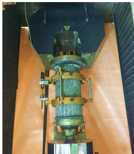
(a) Uniaxial compression test setup
