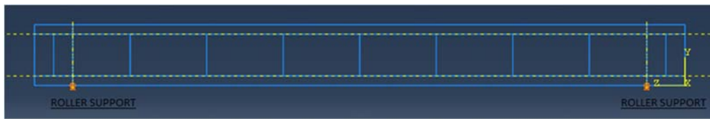
Figure 12: Geometry of a modeled beam and applied boundary conditions.
