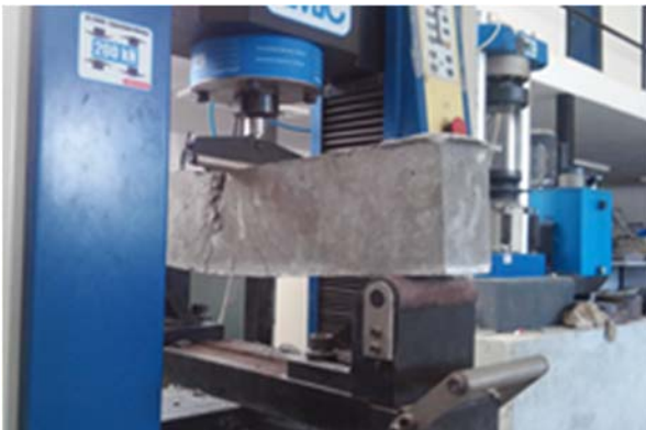
Figure 3: Beam during the test.
