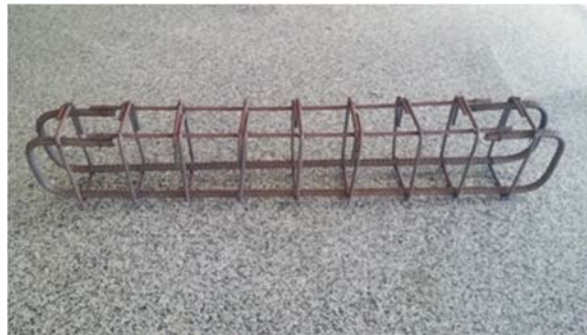
Figure 1: Reinforcement of the beam.
