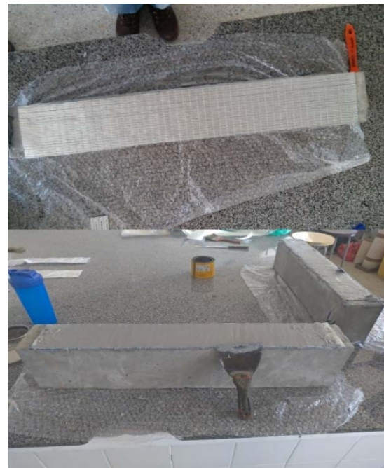
Figure 4: Glass fibre application.
