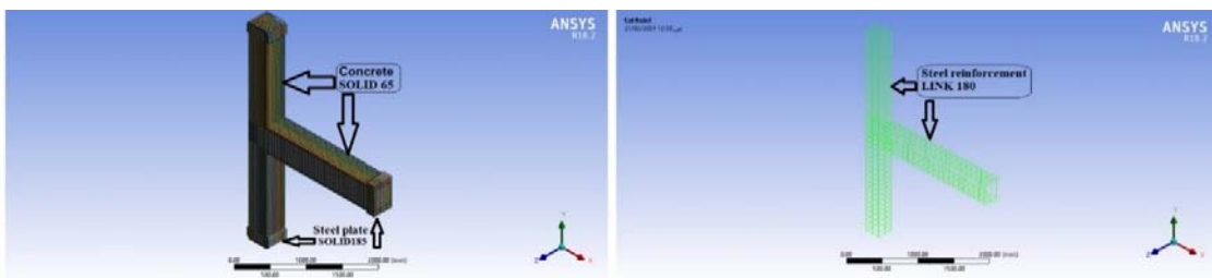
Figure 3: Finite element model details of the studied joint.
