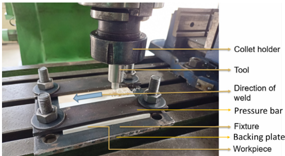
Figure 6: Setup used for the FSW of PLA plates.
