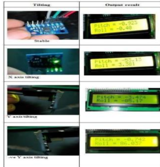
Fig. 10 Output corresponding to tilt of the vehicle
