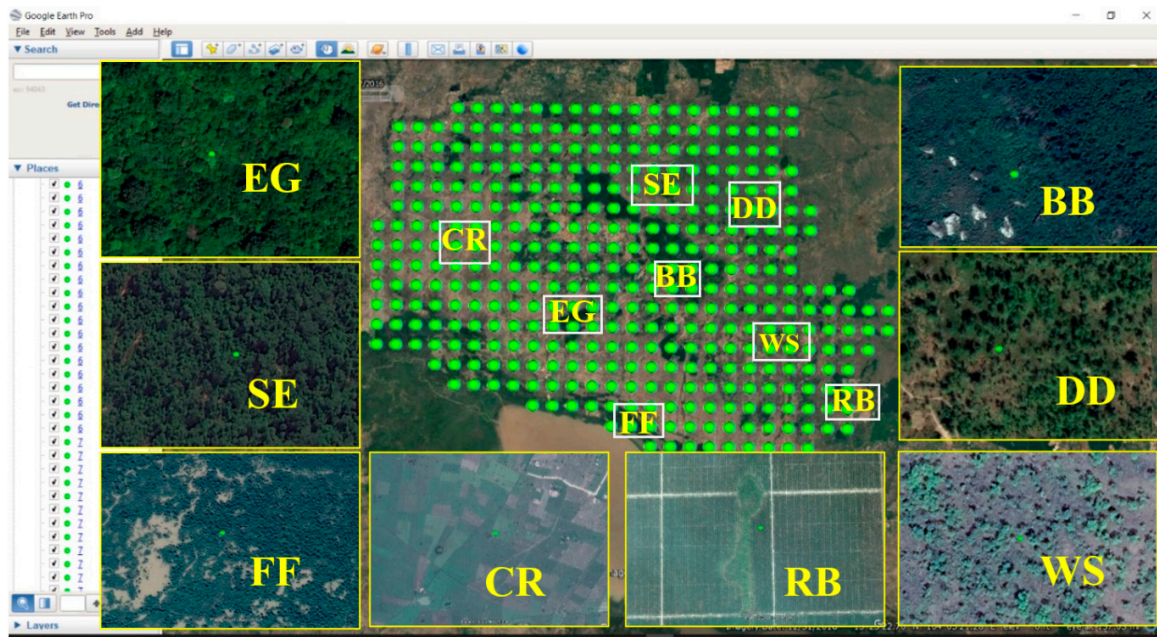
Figure 4. Maps showing the locations of accuracy points for accuracy assessment using Google Earth high-resolution imagery. These points were used to verify and validate the PBTC land cover categories, namely, the Evergreen forest (EG), Semi-Evergreen forest (SE), Deciduous forest (DD), Mixed woods and shrubs (WS), Bamboo (BB), Flooded forest (FF), Rubber plantation (RB), and Croplands (CR).
