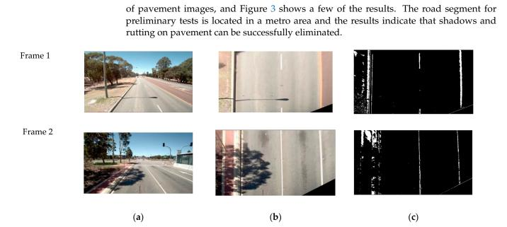
**Figure 3.** Test of the feature extraction method on pavement images. (a) Original images; (b) results of inverse perspective transform; (c) results of feature extraction.
