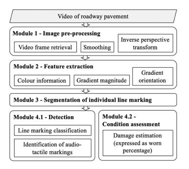
Figure 2. Flowchart of vision-based lane line detection.
