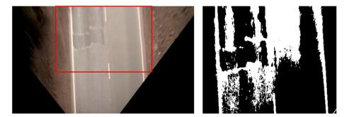
Figure 8. Example of polished pavement.
