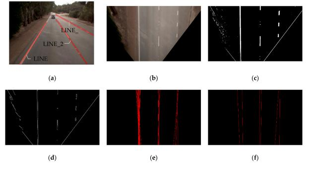
**Figure 7.** Illustrations of image processing steps, including: (a) original image; (b) bird's eye view image; (c) output of hybrid descriptor; (d) output of Canny detector; (e) result of Hough transform; (f) result of segmentation.
