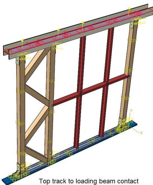
Figure 7.2. Master and slave modelling for contacts of elements in wall panel
