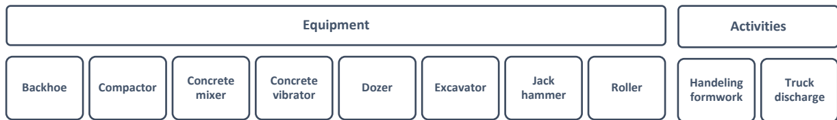
Figure 8.12. Equipment and activities creating pollution during excavation and foundation construction
