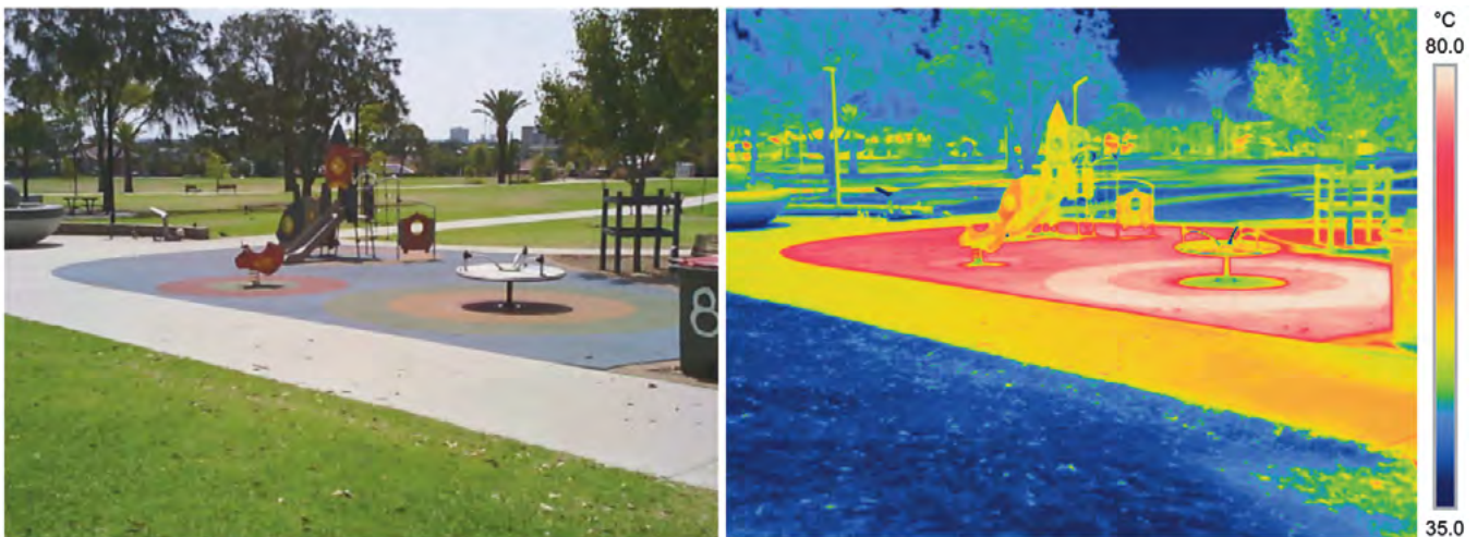
FIGURE 1: Normal (left) and infrared (right) views of the playground at Auburn Park, Auburn. The infrared image shows surface temperature by colour. The colour scale is provided on the right side of the image. Surface temperatures change nearly 50°C within a short distance from the lawn to the playground. Large differences in surface temperature of different materials exposed to the sun are visible (i.e., grass, concrete, different-coloured rubber softfall). The image was taken at 15:00 on 4 January 2020.
