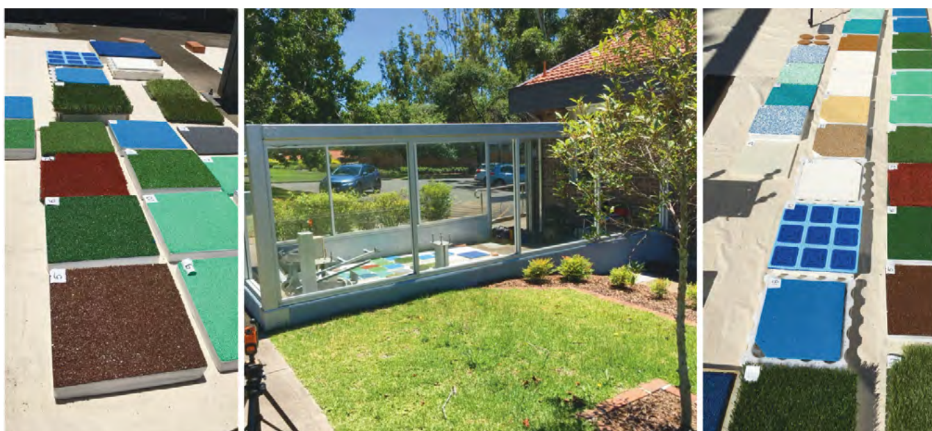
FIGURE 4: Systematic assessment of playground surface materials. The images show a wide range of surface materials, including different rubber softfall materials and colours as well as synthetic turf samples with different pile heights. The materials were exposed to continuous sunshine in a testing facility of the Solar Institute at the Hawkesbury Campus, Western Sydney University, Richmond, NSW.
