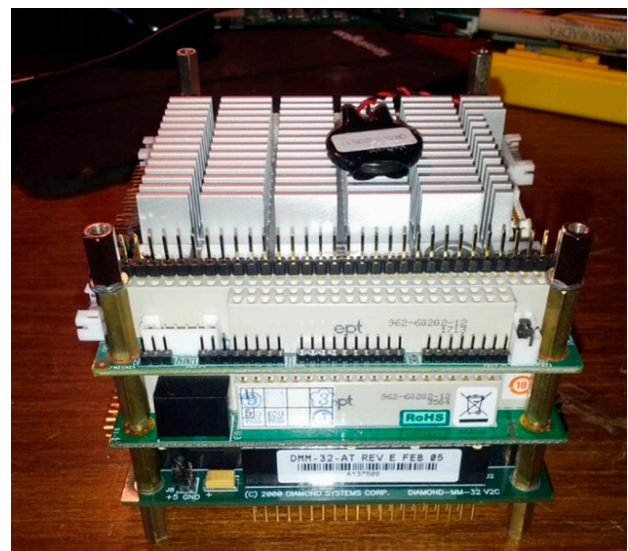
Figure 10: PC104 computer system stack.
