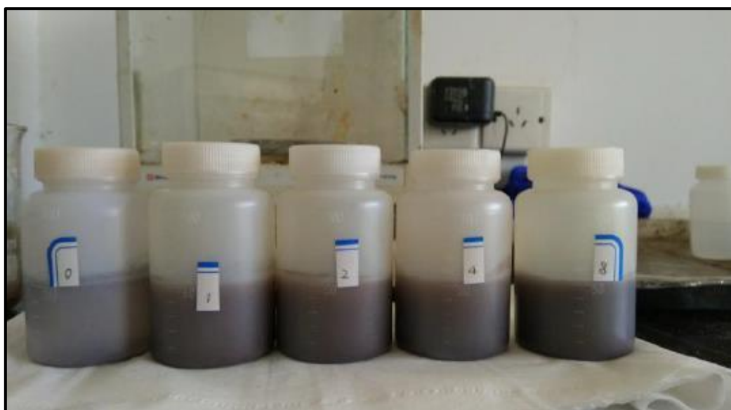
Fig. S3 Photographs for BSMU prepared in the absence/presence of initiator. The results showed that without the initiator the dispersion and stability of the BSMU was not good. The enhanced initiator concentrations enhanced the quality
