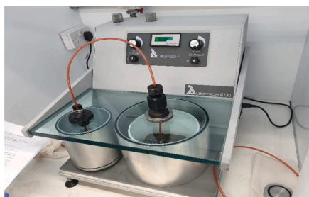
a – Removing air bubbles from sample
